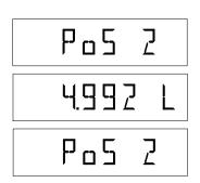
To query PoS 3, press the Up button briefly, then PoS 3 will be shown on the display alternatively with the saved value. If the Up button is pressed again, PoS 4 is displayed, and then if the Up button is pressed again, PoS 5 is displayed.
