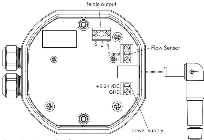
The device and the flow sensor are not protected against overvoltage and polarity reversal.
